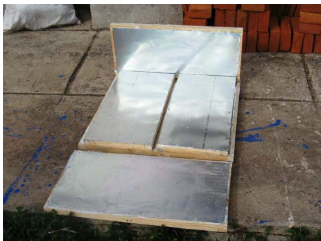
Fig 6: The partly completed portable solar cooker being made in Nicaragua. It will fold down to a packet about 15 cm tall.
