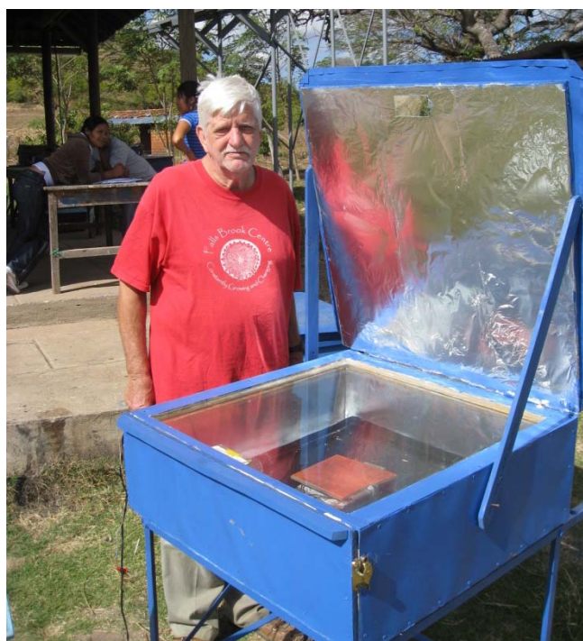
Fig 1 Richard Komp with the solar oven used for laminating the PV modules, showing the clay tile platen used under the module sandwich. This platen has electric heating elements buried in the middle.
