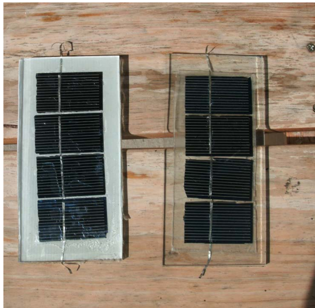
Fig 3 Two small solar battery chargers. The charger on the left with a white PVC back was encapsulated using the two part silicone encapsulant the Solar Women of Totogalpa normally use, while the charger on the right was one of the first modules made with EVA cured in a solar oven. We used a clear PVC plastic backing sheet but didn't make the EVA sheets as big as required.
