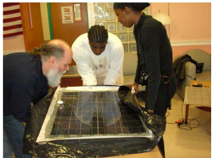
Fig 9 Removing the bubbles from a module being encapsulated at the Addicts Rehabilitation Center in Harlem New York.
