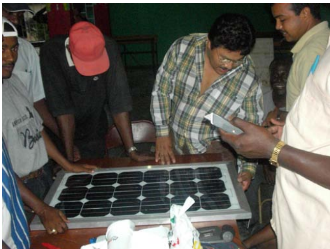
Fig 1 Marco Antonio Perez teaching the first PV module assembly workshop in Haiti in November, 2003. This workshop used the thicker and stronger Astropower single crystal photovoltaic cells.
